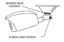
After the correct position has been established, tighten the elbow joint screw and the sensor head locknut at the end of the elbow (near the cover).
